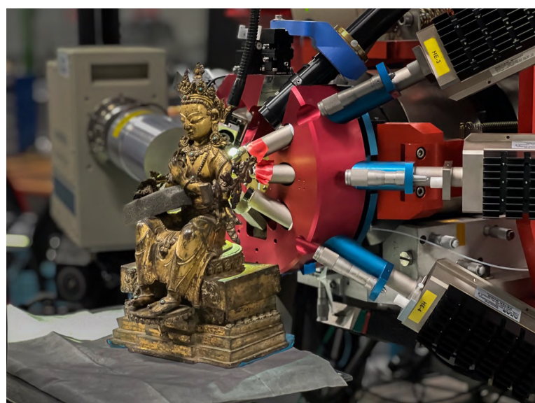
PIXE elemental analysis using the New AGLAE particle accelerator. Analyses: Q. Lemasson, C2RMF. ©C2RMF/A. Lionni.
