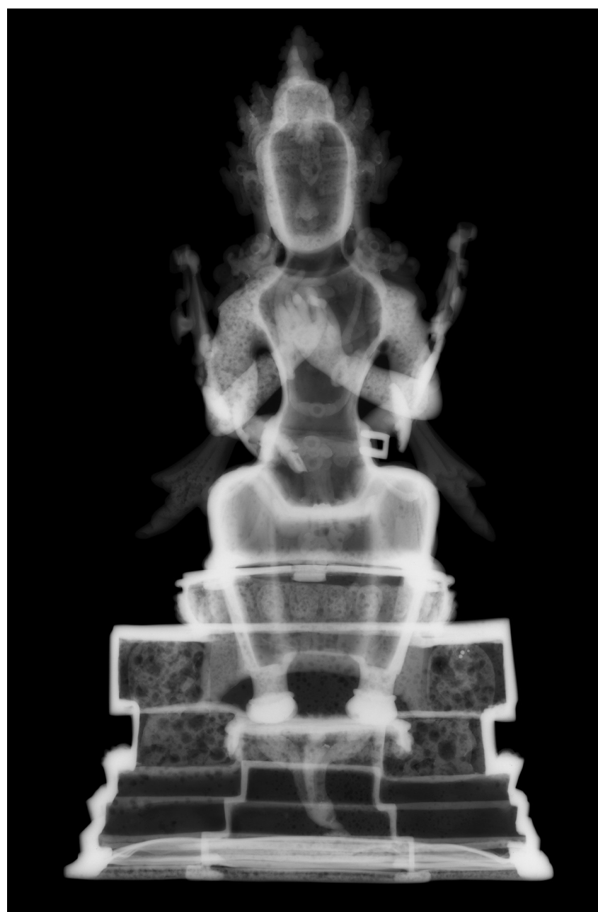
X-radiograph of the statuette showing the hollow structure, casting porosity, and assembly systems. ©C2RMF/E. Lambert.
