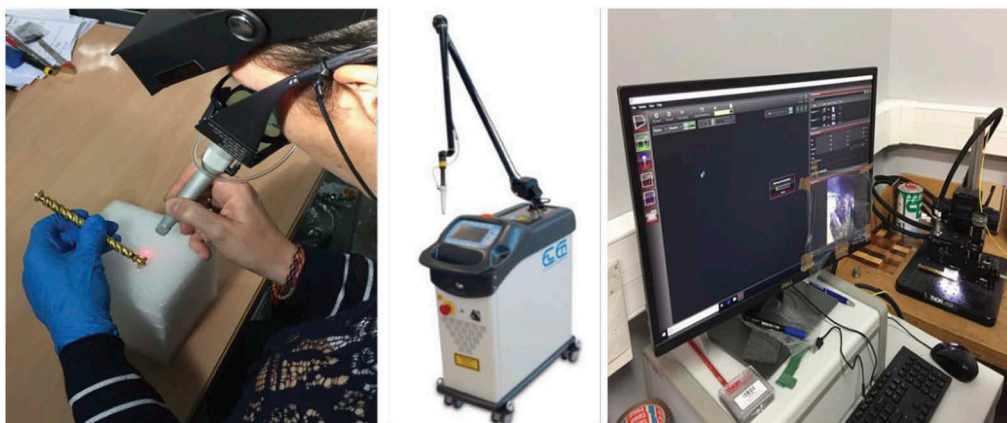
Figure 3. Conservator used the laser on the gilding surface, photographic images of the Laser ER:YAG and Optical Coherence Tomographic (OCT).
